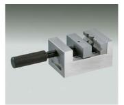
For mounting rectangular and cylindrical workpieces
