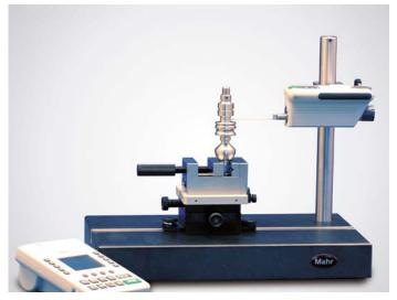
MarSurf measuring station with measuring stand ST-G
