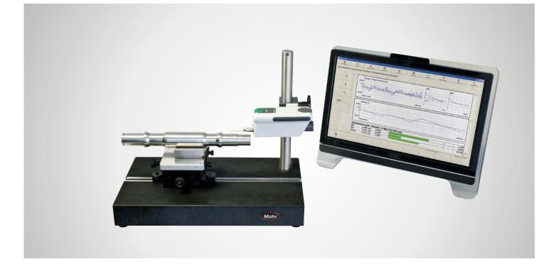
Measuring station for the measurement of roughness depths, P profile and waviness with the drive unit MarSurf SD 26 and the skidless probe system BFW 250.
