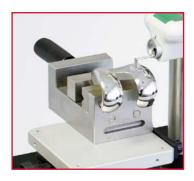
Measurement of a knee joint with drive unit MarSurf RD 18 and skidded probe system PHTR-100
